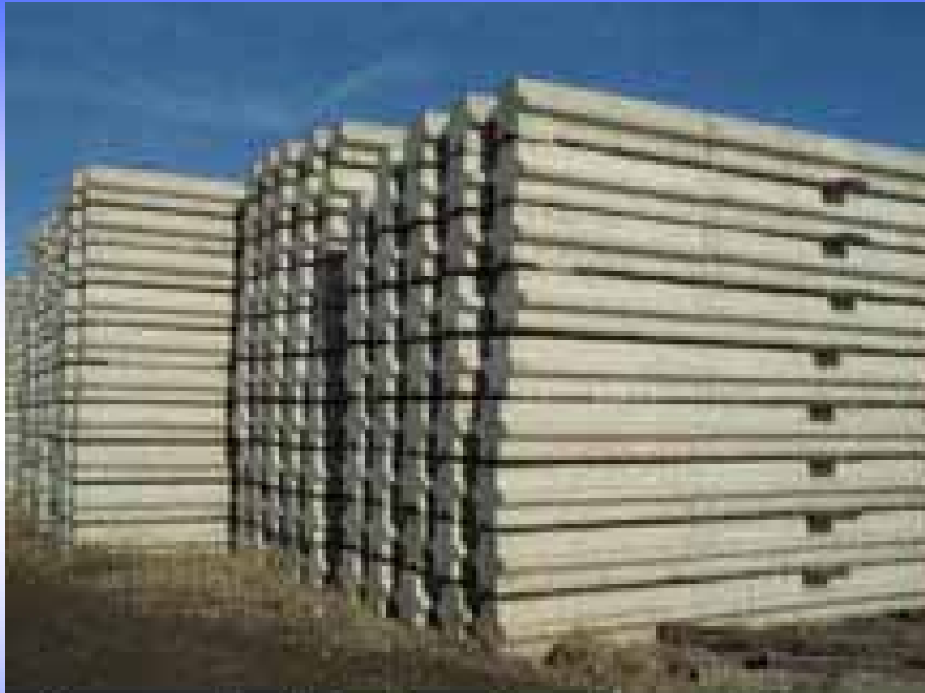
Concrete piles for deep foundations.
